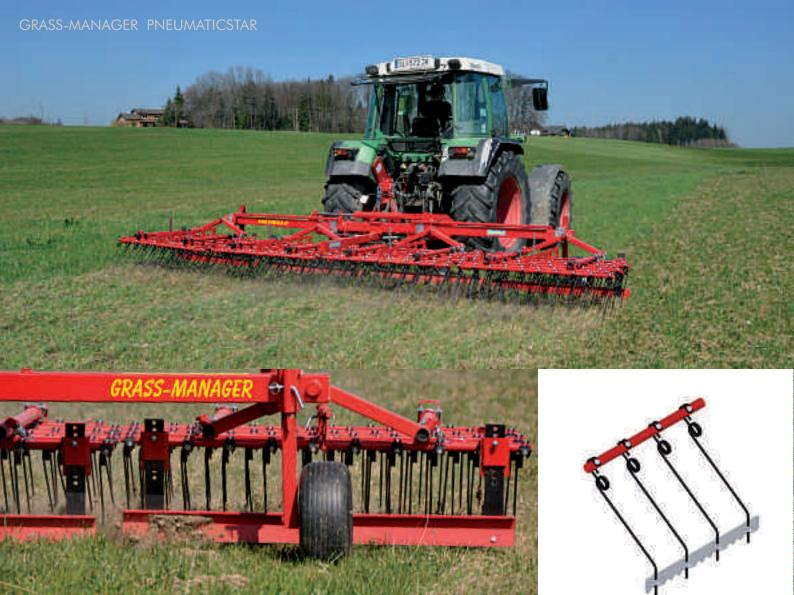
In front of the weeder section a levelling plate can be mounted, which is overload-protected by a leaf spring. This **levelling plate** is height adjustable and ensures an excellent **distribution and levelling of molehills**. In addition, it distributes and levels manure and slurry. It can easily be retro-fitted.
