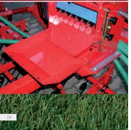
The **calibration pan** and cover are standard on the machines.
