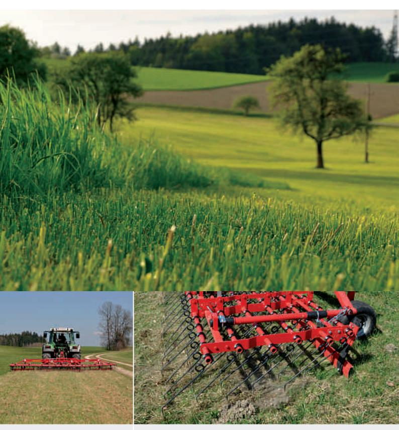
The **6 row weeder section** carries 60 tines on 1.5 m working width; this equals a **line spacing of 2.5 cm**. This narrow line distance ensures a good effect in dethatching of the soil and excellent result.
