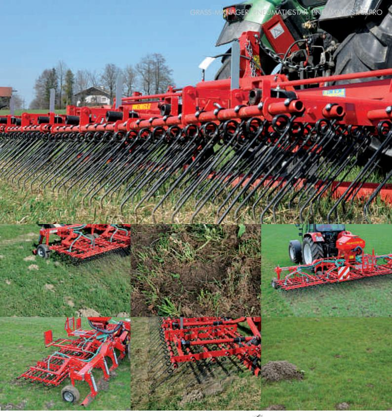
In **heavily felted grassland** or extremely heavy soil, tines with 10 mm diameter and 490 mm length must be used. These tines are ideal to **fight rough stalked meadow grass** in summer.
