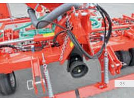
The Farmflex rubber roller, depth adjustable via a breadboard and with 520 mm ø, ensures an **optimal reconsolidation**.
