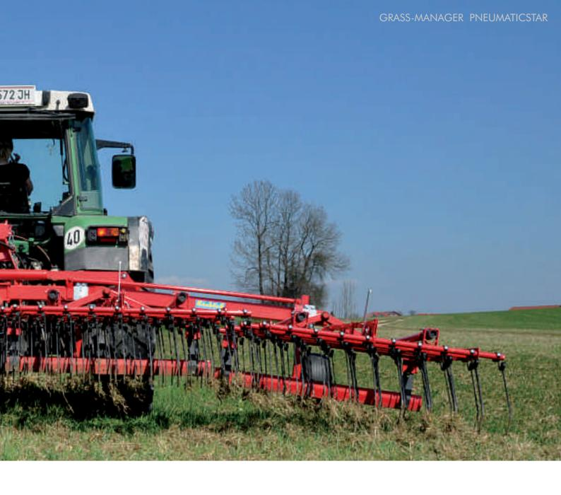
By taking away or mounting of the stop bar on the wing (only on machines without shear retraction) the machine **follows the contours of the land surface** perfectly.
