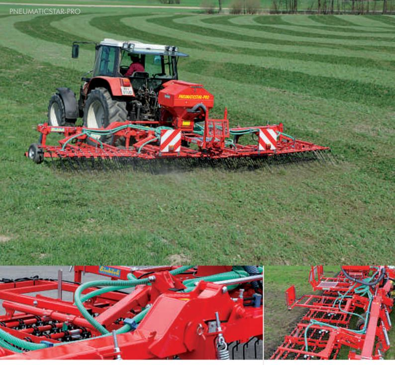
The joints consist of a **hardened bolt** with 35 mm Ø and brass bushings which can be greased.
