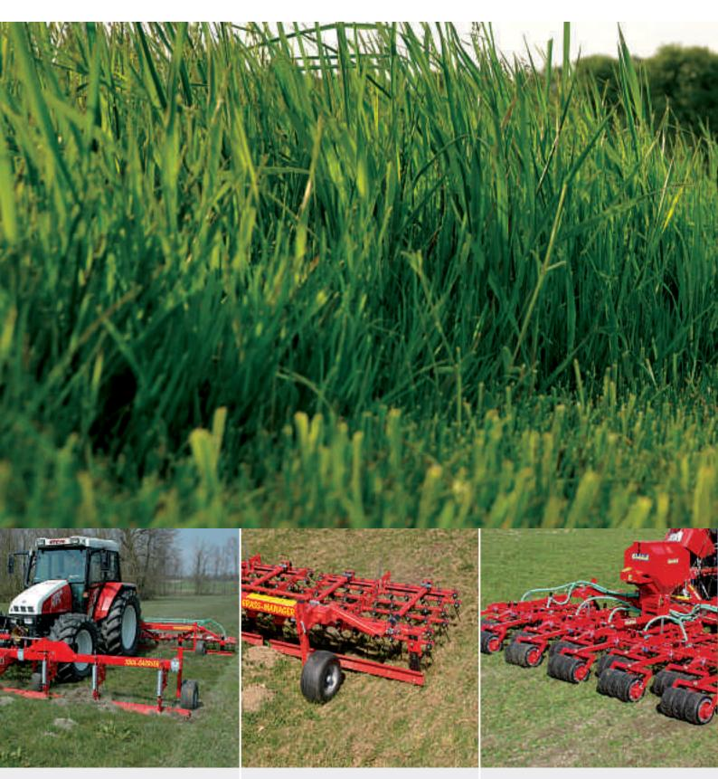
The **front mounted TOOL-CARRIER**, like the PNEUMATICSTAR-PRO, is equipped with heavy levelling boards. For clients, who have a lot of molehills and already own a GRASS-MANAGER or PNEUMATICSTAR, the TOOL-CARRIER is a real alternative. This machine is designed for the front linkage and has a working width of 6m.
