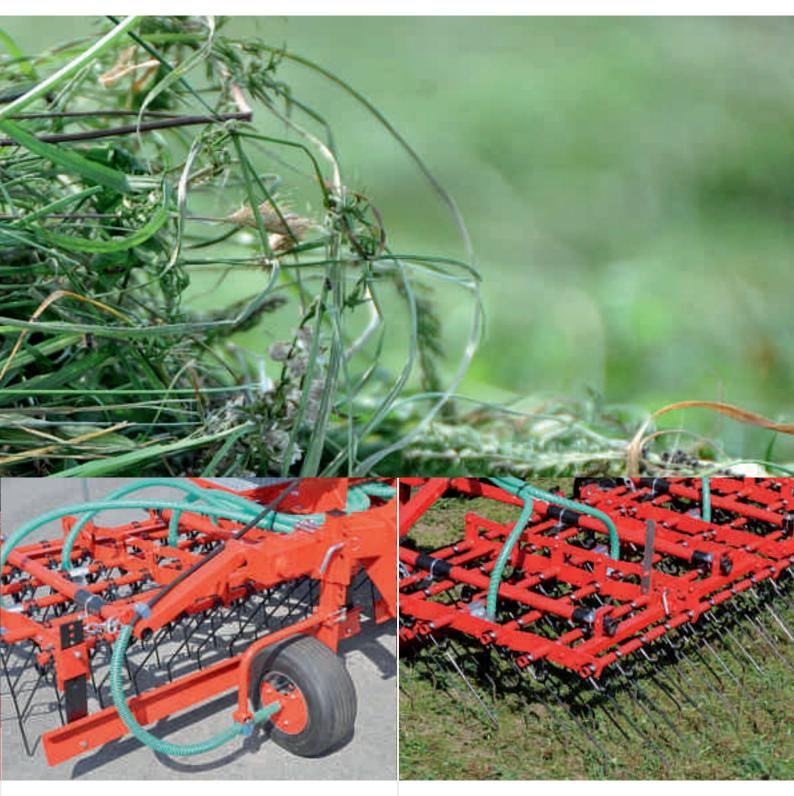
**Ground drive** via the support wheel (PNEUMATICSTAR). The flexible shaft, which runs a stepless oil bath gearbox, is protected by a hose. The information about working speed is provided by the support wheel. There is no additional ground wheel necessary.
