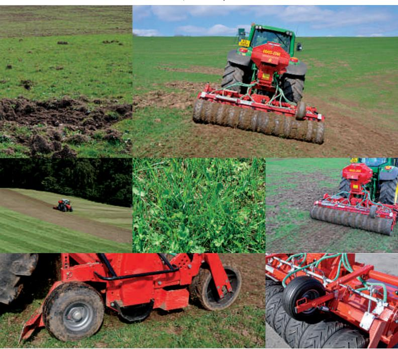
**Scraper boards** level the soil in front of the support wheels which care for an exact depth guidance.
