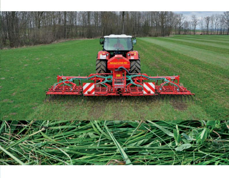
The **tine aggresiveness** can be adjusted by a **central lever** per section in 5 positions. On "hold" adjusted tines have a stronger de-thatching effect and fight the rough stalked meadow grass very effectively.
