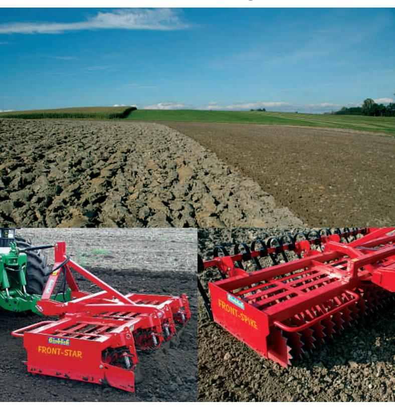
The FRONT-STAR is especially designed for heavy and soggy soils. It is equipped with a spring loaded, height adjustable leveling plate, which makes a first leveling and crushing of the soil. After this leveling board the 3-rows of star-discs follow; due to their special design they crush the clods without clogging.
