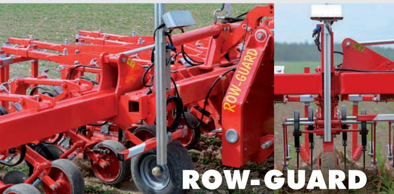
The camera steering system ROW-GUARD steers inter-row crop cultivators precisely between the rows and supports the operator. The tractor driver only needs to concentrate on driving in the correct row, the exact guidance of the cultivator is done by the precision steering system.
