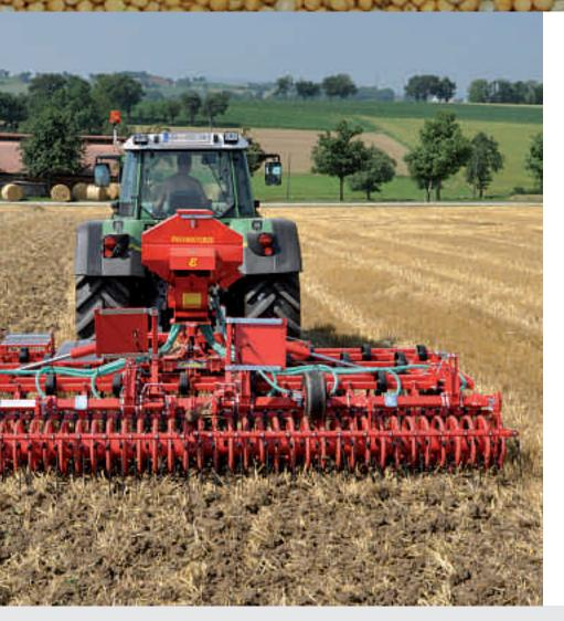
With the pneumatic air seeder PNEUMATICBOX many different kinds of seeds can be distributed.
