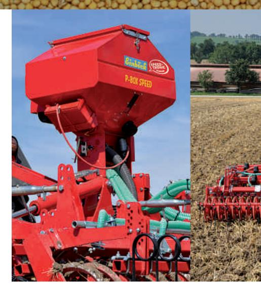
For an exact seeding rate also in changing working speed the P-BOX SPEED can be equipped with the SPEED-TRONIC control unit. The 7-pin plug of the tractor, a wheel or a radarsensor provide the necessary information about the working speed.
