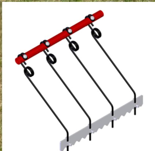
In front of the weeder section a levelling plate can be mounted, which is overload-protected by a leaf spring. This **levelling plate** is height adjustable and ensures an excellent **distribution and levelling of molehills**. In addition, it distributes and levels manure and slurry. It can easily be retro-fitted.
