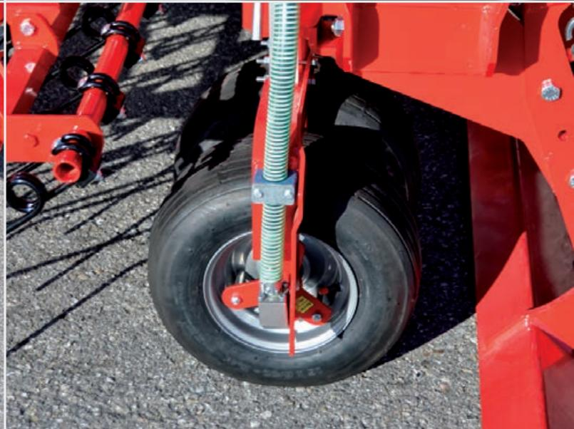
**Ground drive** via the support wheel (PNEUMATICSTAR). The flexible shaft, which runs an infinitely variable oil bath gearbox, is protected by a hose. The information about working speed is provided from the support wheel. There is no additional ground wheel necessary.
