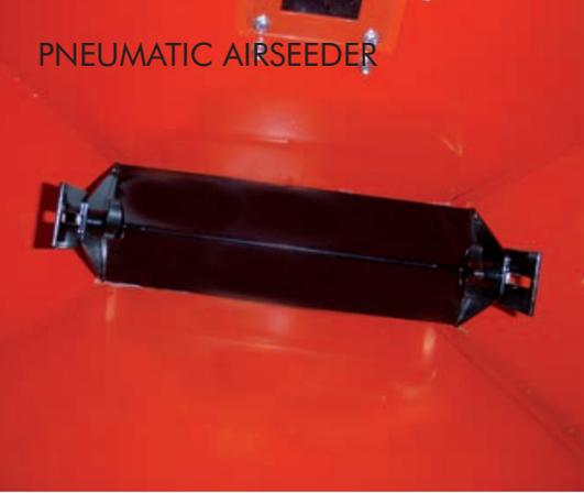
For heavy seeds we recommend a **retaining plate**, which is mounted on top of the stirring shaft and the seeding roller.
