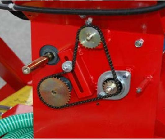
A **chain with tensioner** connects the infinitely variable oil bath gearbox (or the electric seeding roller motor) with the seeding roller and the stirring shaft.
