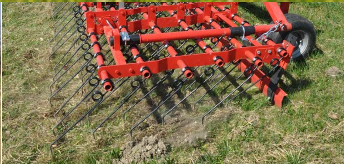
■ The **6 row weeder section** carries 60 tines on 1.5 m working width; this equals a **line spacing of 2.5 cm**. This narrow line distance ensures a good effect in dethatching of the soil and excellent result.
