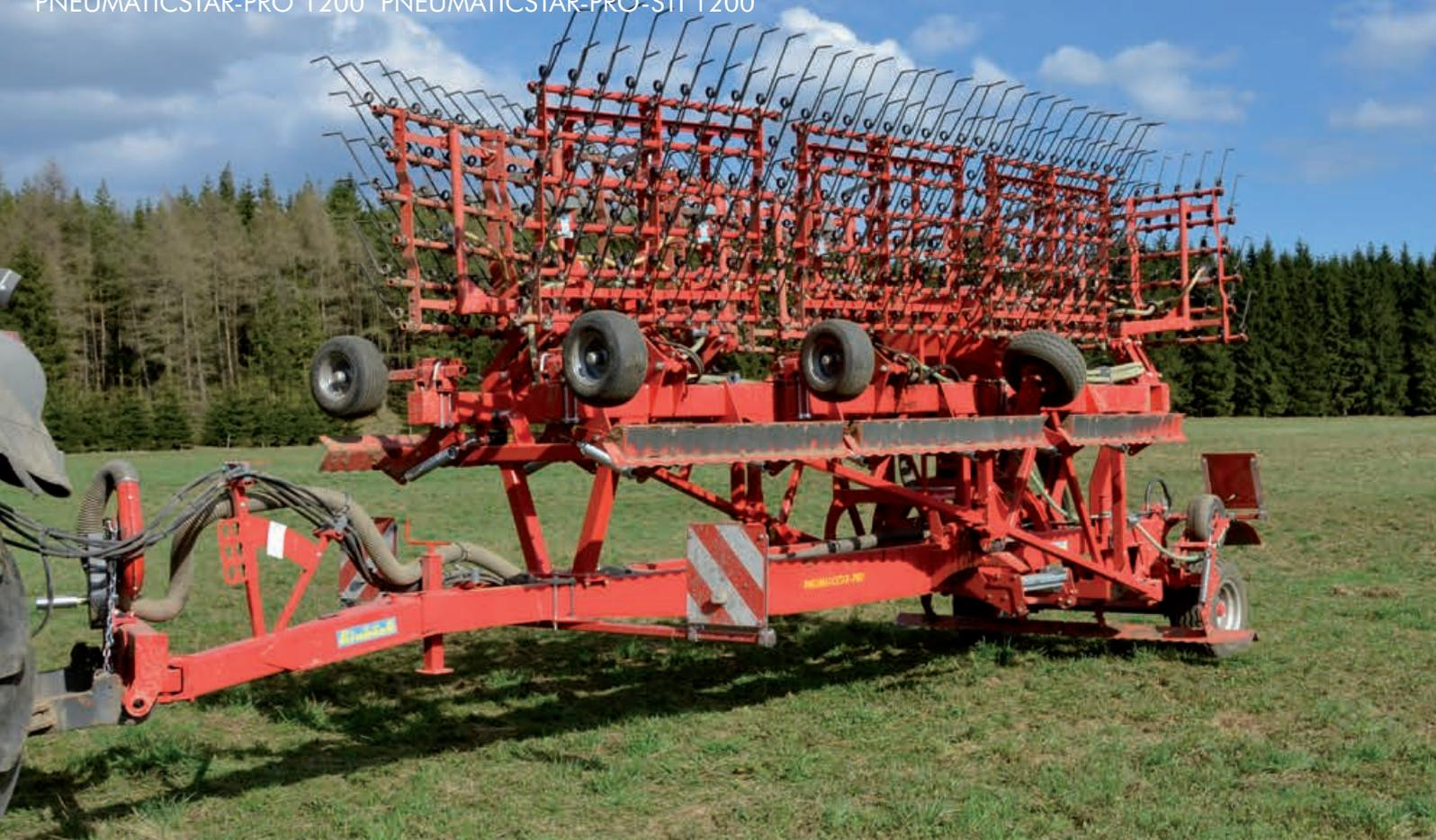
The sophisticated **retraction mechanism** together with putting the tines into the lowest angle position makes it possible to reduce the transport width to only 3 m
