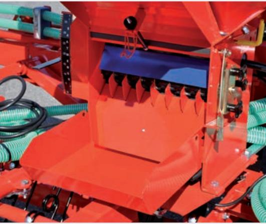
The **calibration pan** and cover are standard on the machines.
