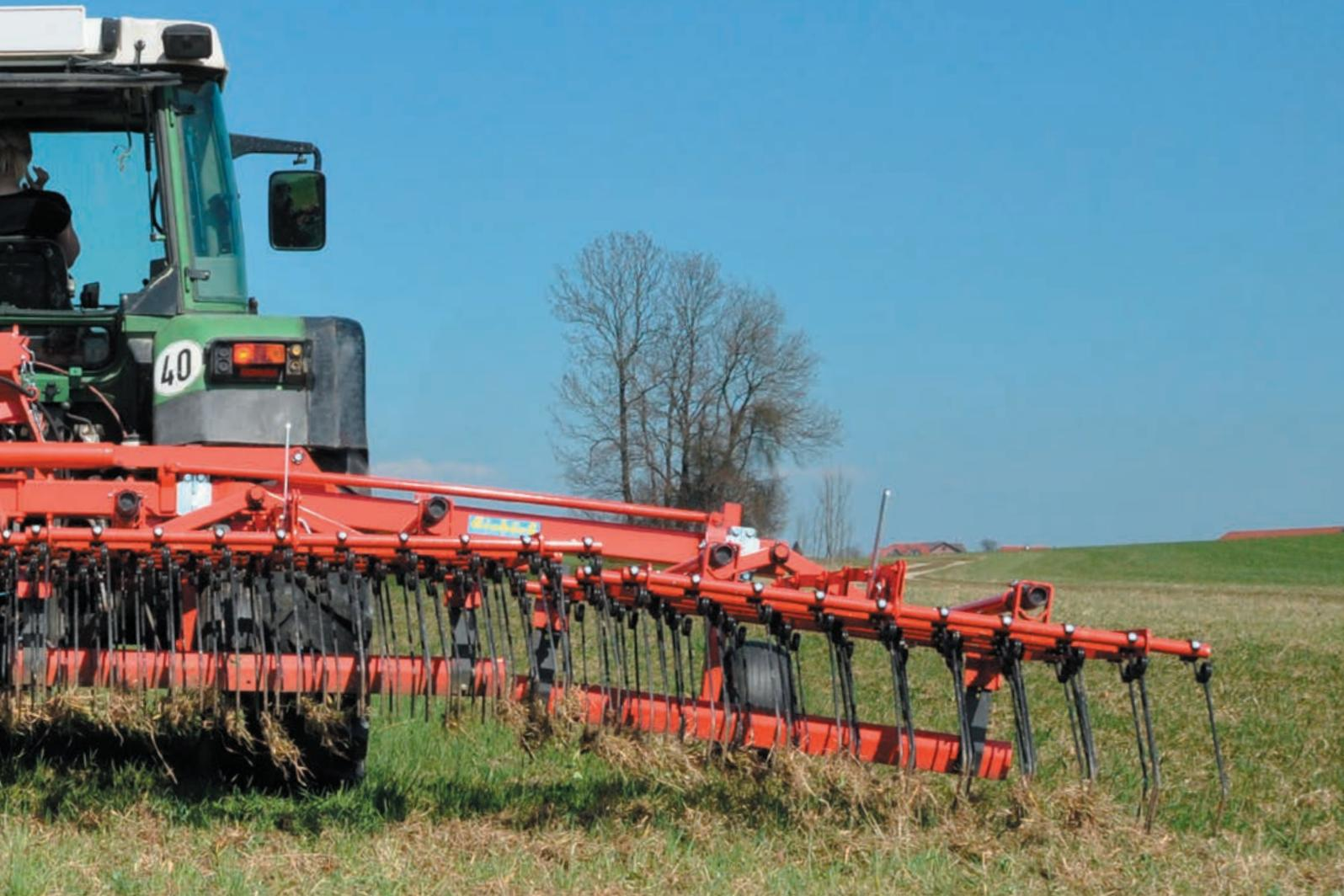
■ By taking away or demounting the stop bar on the wing (only on machines without shear folding) the machine **follows the contours of the land surface perfectly**.
