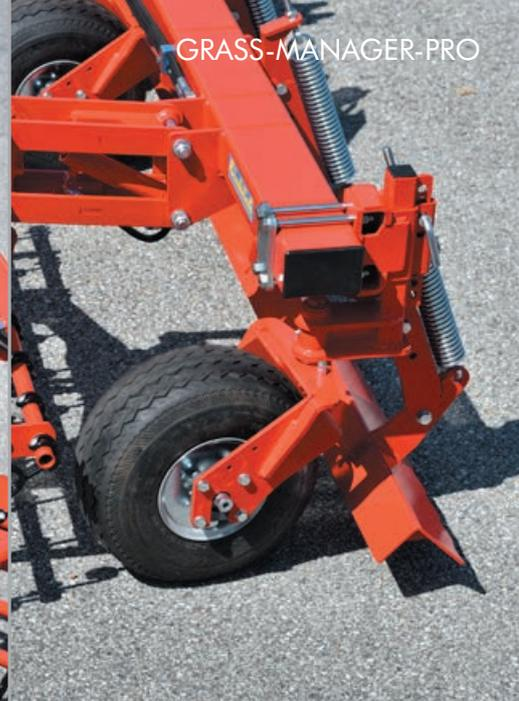
For the PRO-series there is a **front mounting frame** available. With this frame an existing rear mounted machine can easily be converted into a front mounted machine.
