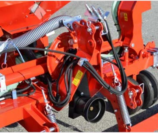
With the **mechanical fan** you can distribute heavier seeds up to 6 m working width due to the higher airstream. You can work with increased working speed. Recommended for communities and contractors.
