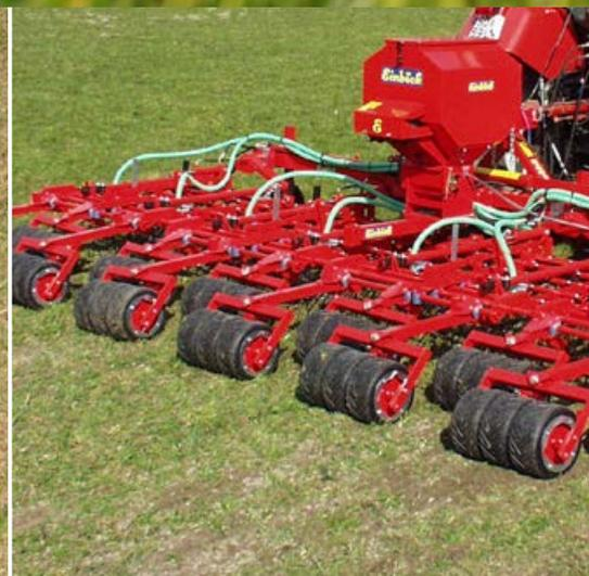
The PNEUMATICSTAR and the PNEUMATICSTAR-STI are available with **reconsolidation rolls**. These are made from FARMFLEX-rubber and cannot get stuck with soil. The rolls are mainly used for new seeding or to re-seed large gaps in the turf to establish seed/soil contact. The short pressing rolls (3 units for every 1.5 m working width) with axle-pendular mounting follow the surface of the turf precisely.
