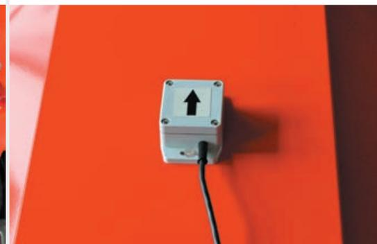
The **tank level sensor** signalizes, when the tank is getting empty. The sensor works inductively, therefore it is vibration independent.
