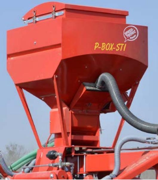
On request the airseeders are available with a **500 litres seed tank** (with tank support and extra-large opening).
