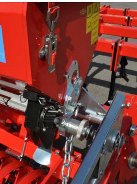
The DRILLBOX/MECHANICBOX is suitable for the use on rigid tilling implements. In a very easy and solid way you can seed 5 kg/ha of any intercrop seed and seed mix in a simple oversowing procedure using a knob for fine and a lever for coarse settings. The seedbox features an activation wheel system with baffle plates and can also be equipped with a stirring shaft for an extra charge.
