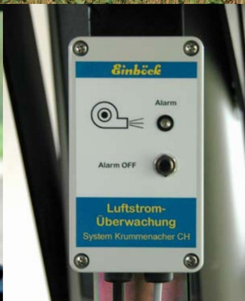
With **this control unit**, that can easily be mounted in the tractor cabin with a velcro, you can switch on/off the electric fan.
