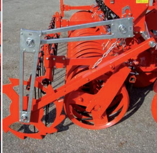
The **arm of the bottom drive wheel** is adjustable in length. Because of its large diameter of 600 mm the drive wheel grants an exact activation of the shearing wheels also in rough terrain.
