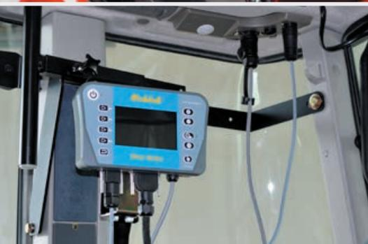
The **linkage sensor** turns off the seeding roller when the machine is lifted up.
