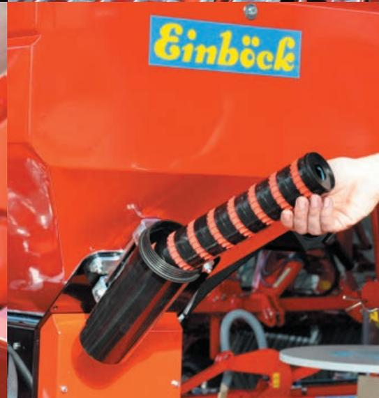
The **seeding roller** distributes the seeds into the eight divided and separated outlets. From there it is transported pneumatically via the PVC seed hoses to the deflector plates from where it is exactly spread over the entire working width. Since the seeds are blown pneumatically, wind does not matter as much as it would with mechanical seeders.
