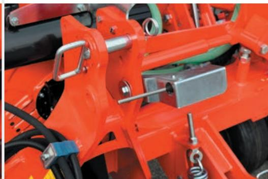
The sensors of the **airflow monitoring** signalize, whether one or more seeding hoses are clogged.
