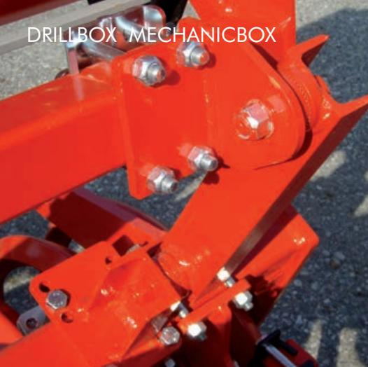
The **mounting consoles**, which can be adjusted in an angle by a toothed wheel fit to 60, 70, 80, 90 and 100 mm steel tubes.
