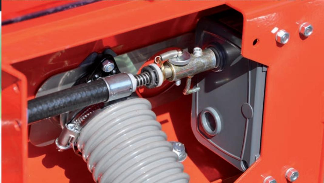
In case there are areas you do not want to seed, you can disconnect the flexible shaft from the gearbox by **taking away the bolt** where the shaft enters the gearbox.
