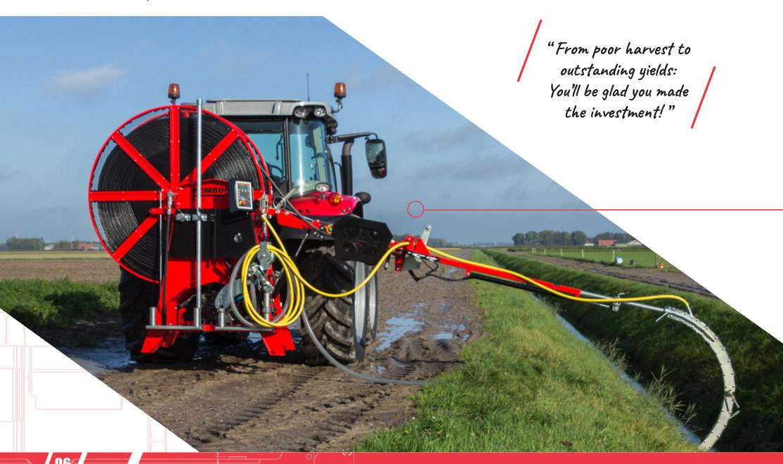
The DELTA offers more ease of use as a draincleaner than the JUNIOR. This is the ideal machine for anyone who maintains drainage systems on a frequent basis and needs to cover a large area. This is because it offers hydraulically operated height adjustment, extension, retraction and folding of the drainage arm and length adjustment of the guide arm.
