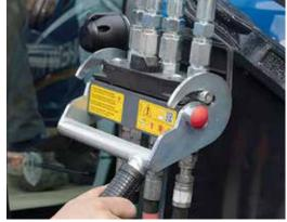
With the Hydro-Fix all hydraulic lines can be connected to the tractor at the same time. The front loader is lifted slightly to hold the locking pin in position in the catch hook of the connection support.
