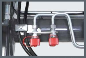
Using hydraulic implements effectively – thanks to the third pilot circuit, there is no need for an additional control unit.
