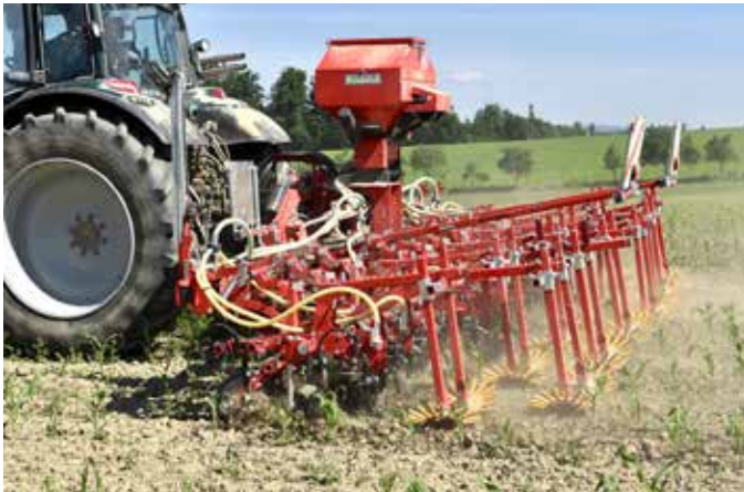
Undersowing in corn with a row-crop cultivator
