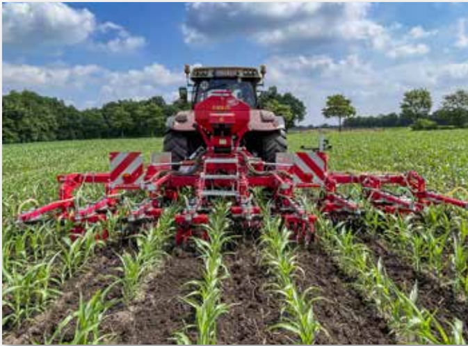
Undersowing in corn with a row-crop cultivator
