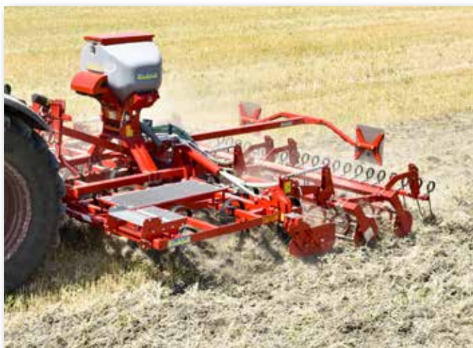
Seeding cover crops with a blade cultivator
