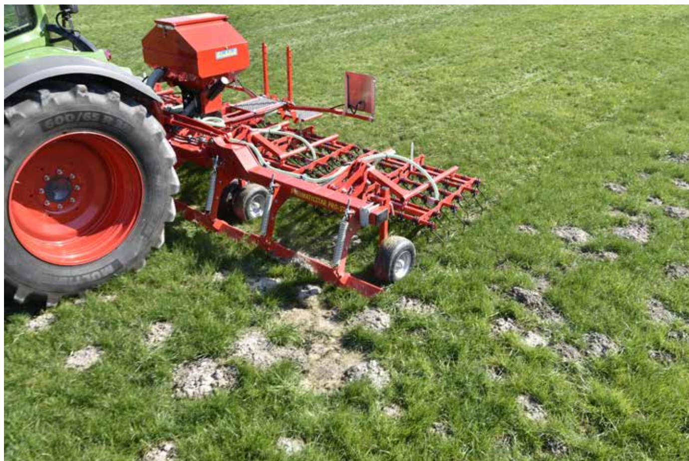
Well-managed grassland with a low amount of rough meadow-grass. During a pass carried out as part of the spring maintenance, the sward is aerated, molehills are levelled off and seeds are oversown.
